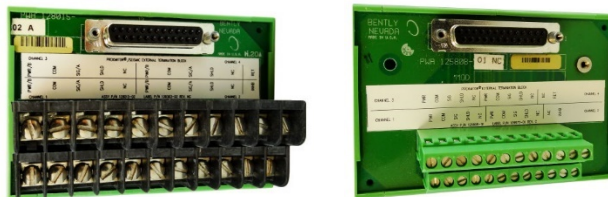
Figure 7: ET Blocks with screw terminals for lugged field wiring (left) and high-density “Euro” connectors for non-lugged field wiring (right)
